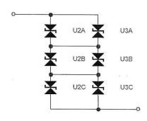
It is composed of 3 series elements of SMDMAX15KA-66CA and this combination will provide a protection of 360v for an 8/20 pulse of 30 kA.
